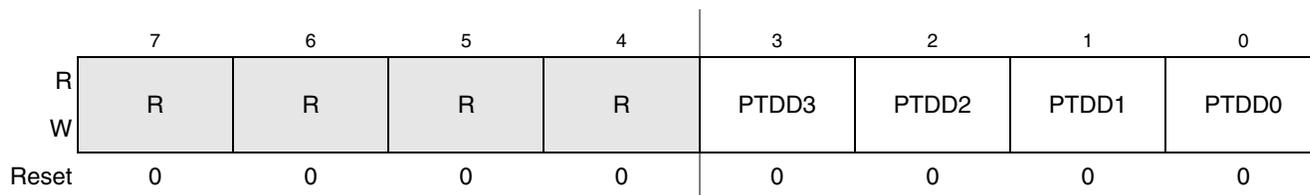
**Figure 6-25. Port D Data Register (PTDD)<sup>1</sup>**
