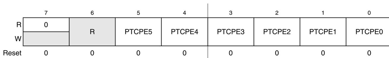
**Figure 6-22. Internal Pullup Enable for Port C (PTCPE)<sup>1</sup>**
