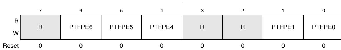
**Figure 6-37. Internal Pullup Enable for Port F (PTFPE)<sup>1</sup>**
