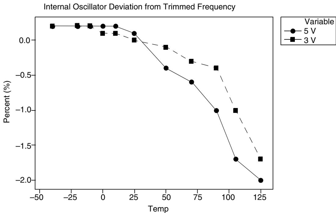
Device trimmed at 25°C at 3.0 V.
