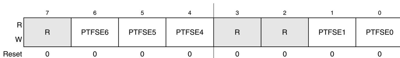
**Figure 6-38. Output Slew Rate Control Enable for Port F (PTFSE)<sup>1</sup>**
