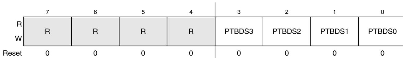
**Figure 6-19. Output Drive Strength Selection for Port B (PTBDS)<sup>1</sup>**
