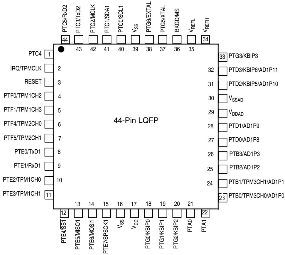
Figure 2-2. MC9S08AC16 Series in 44-Pin LQFP Package
