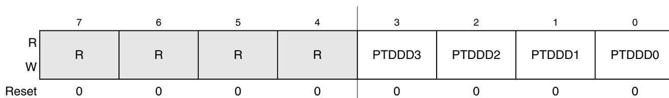
**Figure 6-26. Data Direction for Port D (PTDDD)<sup>1</sup>**
