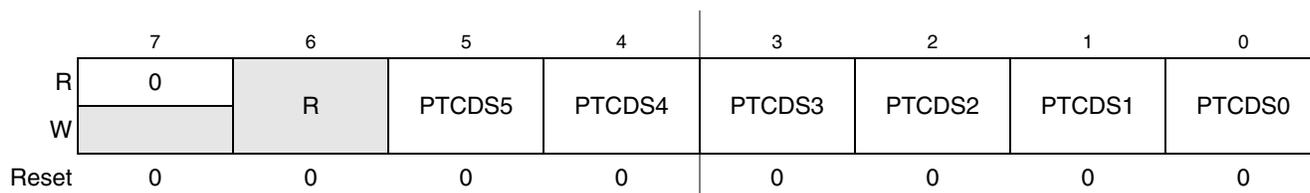
**Figure 6-24. Output Drive Strength Selection for Port C (PTCDS)<sup>1</sup>**
