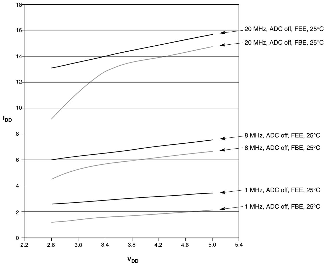
**Note:** External clock is square wave supplied by function generator. For FEE mode, external reference frequency is 4
