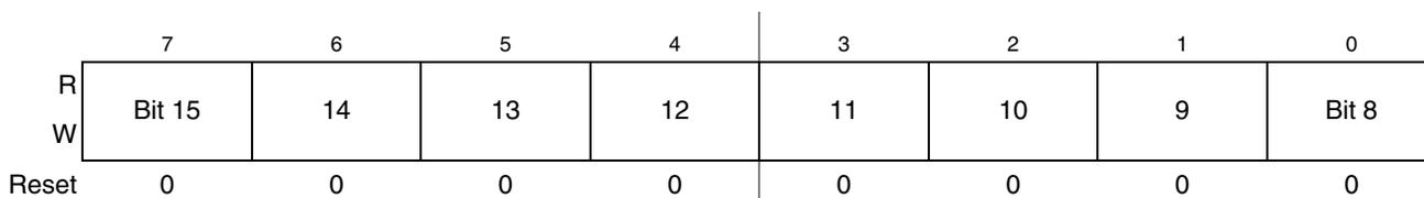
**Figure 10-13. TPM Channel Value Register High (TPMxCnVH)**
