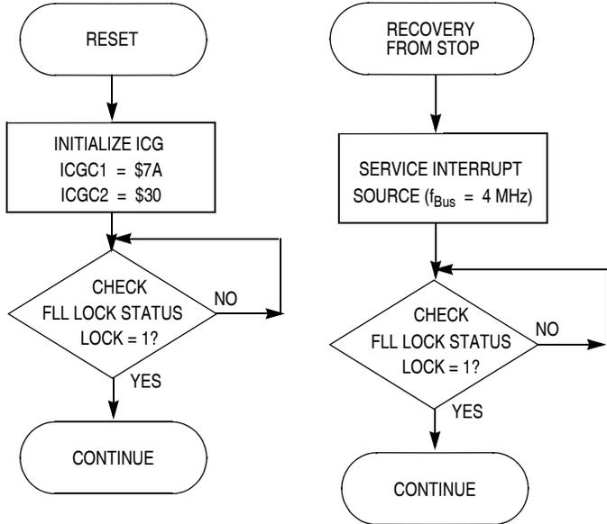
Figure 8-15. ICG Initialization and Stop Recovery for Example #2
