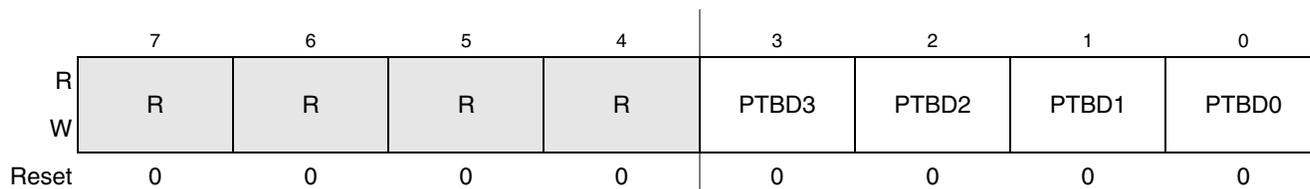
**Figure 6-15. Port B Data Register (PTBD)<sup>1</sup>**
