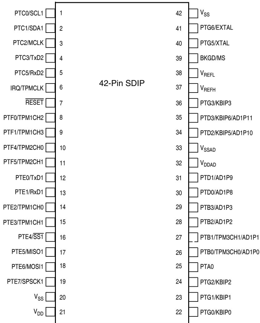
Figure 2-3. MC9S08AC16 Series in 42-Pin SDIP Package
