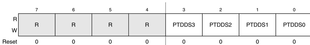
**Figure 6-29. Output Drive Strength Selection for Port D (PTDDS)<sup>1</sup>**
