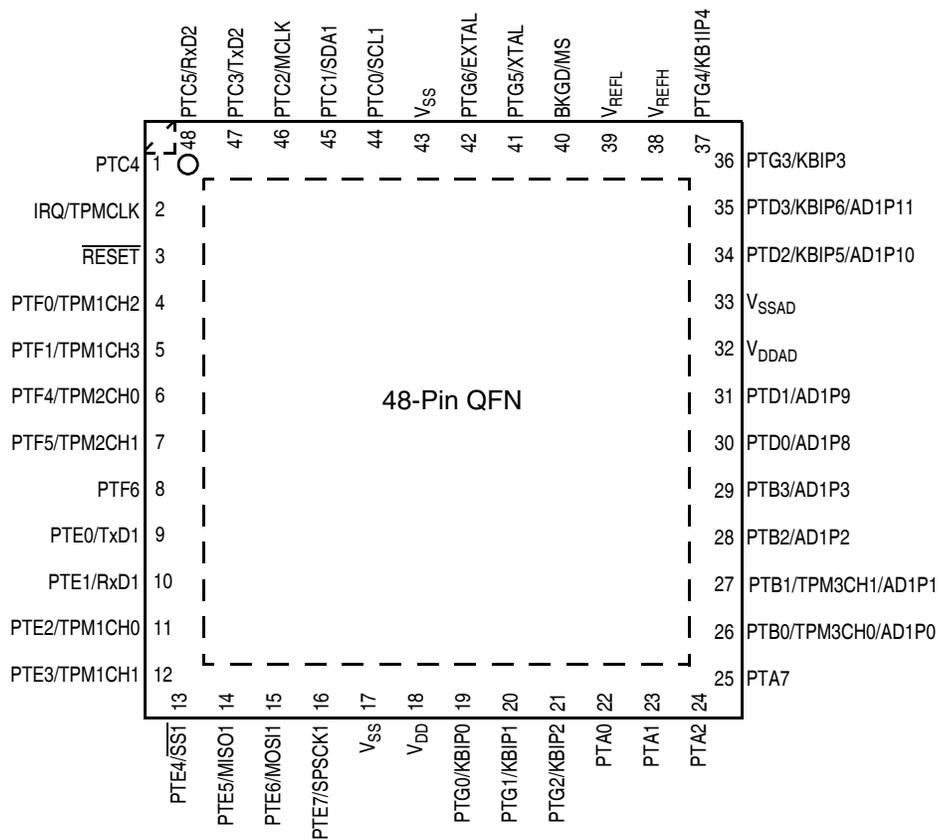
Figure 2-1. MC9S08AC16 Series in 48-Pin QFN Package
