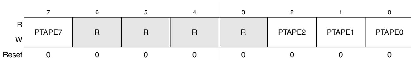
Figure 6-12. Internal Pullup Enable for Port A (PTAPE)<sup>1</sup>
