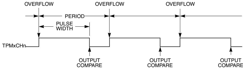
**Figure 10-15. PWM Period and Pulse Width (ELSnA=0)**
