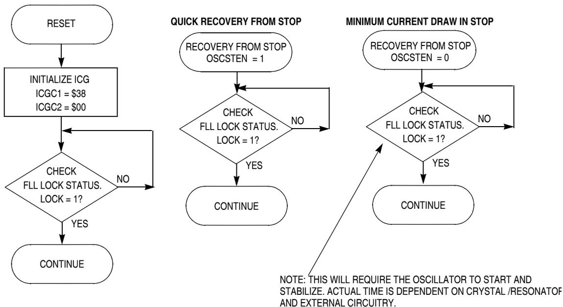
Figure 8-14. ICG Initialization for FEE in Example #1
