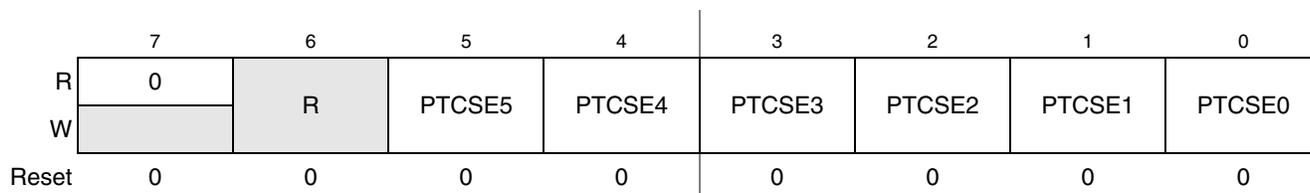
**Figure 6-23. Output Slew Rate Control Enable for Port C (PTCSE)<sup>1</sup>**
