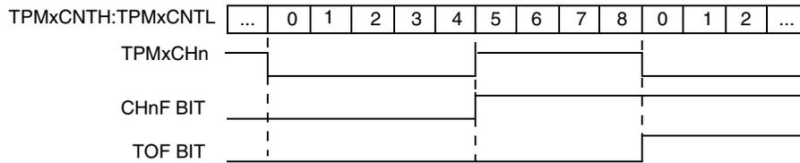
**Figure 10-4. Low-True Pulse of an Edge-Aligned PWM**
