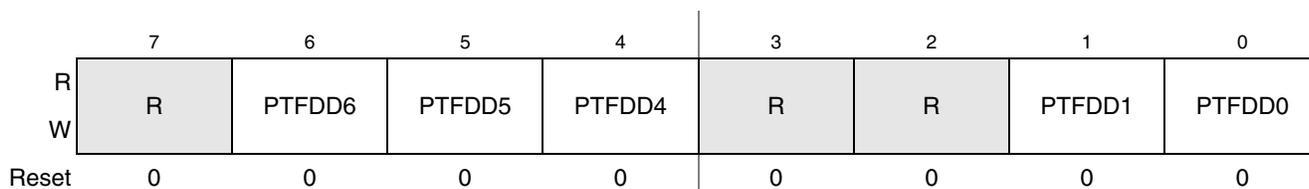
**Figure 6-36. Data Direction for Port F (PTFDD)<sup>1</sup>**
