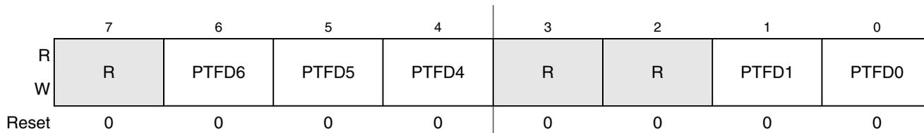
**Figure 6-35. Port F Data Register (PTFD)<sup>1</sup>**
