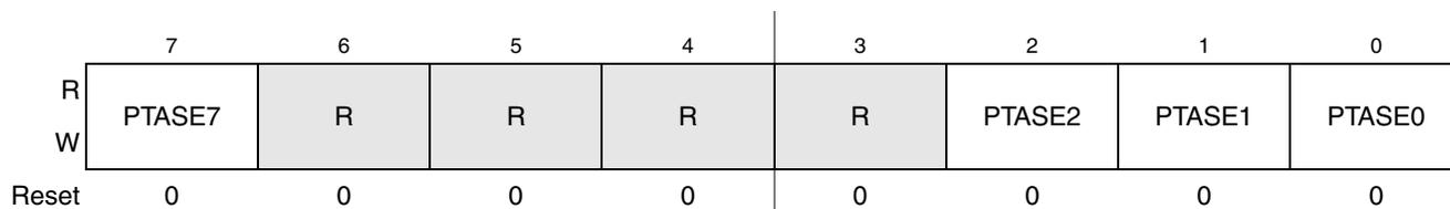
**Figure 6-13. Output Slew Rate Control Enable for Port A (PTASE)<sup>1</sup>**
