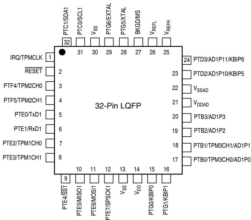
Figure 2-4. MC9S08AC16 Series in 32-Pin LQFP Package
