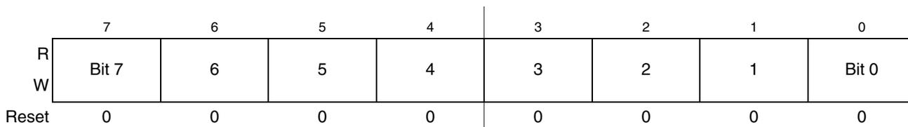
**Figure 10-14. TPM Channel Value Register Low (TPMxCnVL)**
