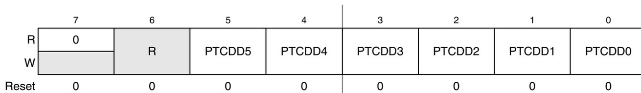
**Figure 6-21. Data Direction for Port C (PTCDD)<sup>1</sup>**
