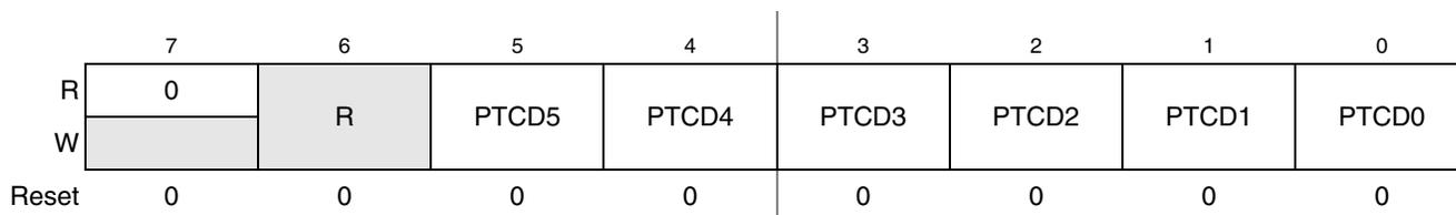
**Figure 6-20. Port C Data Register (PTCD)<sup>1</sup>**
