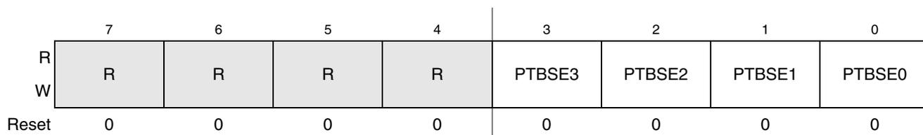
**Figure 6-18. Output Slew Rate Control Enable (PTBSE)<sup>1</sup>**
