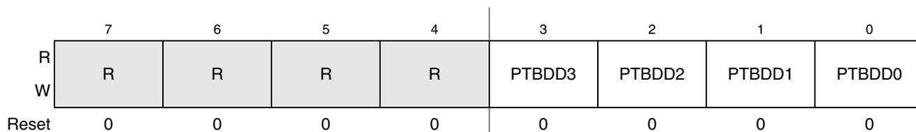
**Figure 6-16. Data Direction for Port B (PTBDD)<sup>1</sup>**
