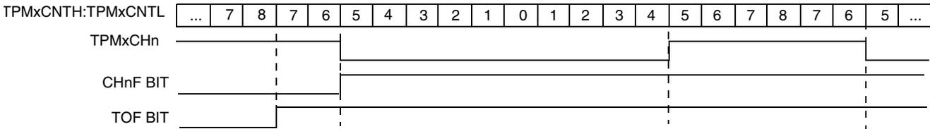
Figure 10-6. Low-True Pulse of a Center-Aligned PWM
