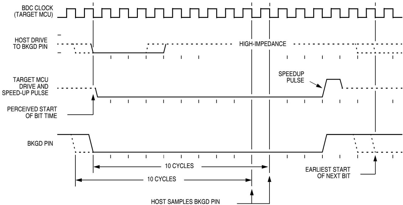
**Figure 15-4. BDM Target-to-Host Serial Bit Timing (Logic 0)**
