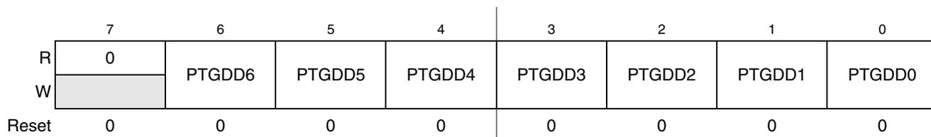
Figure 6-41. Data Direction for Port G (PTGDD)
