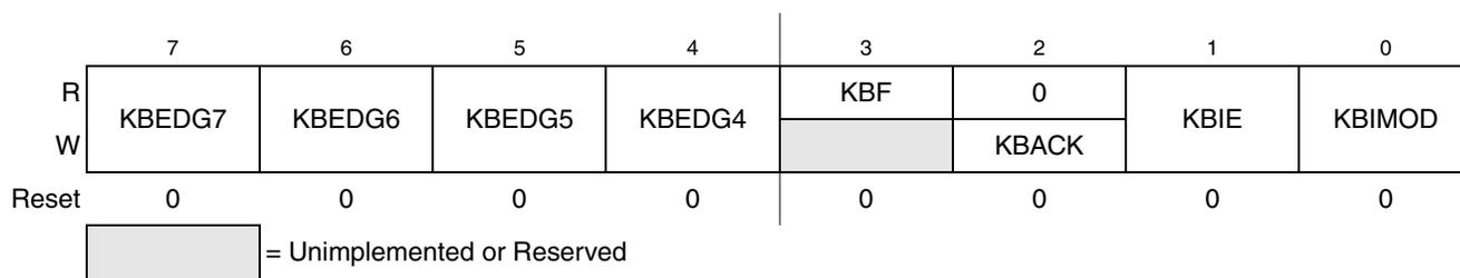
**Figure 9-3. KBI Status and Control Register (KBISC)**
