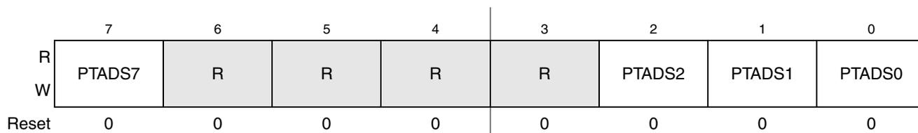
**Figure 6-14. Output Drive Strength Selection for Port A (PTADS)<sup>1</sup>**
