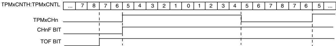
Figure 10-5. High-True Pulse of a Center-Aligned PWM
