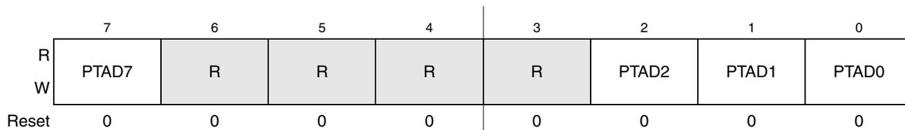
**Figure 6-10. Port A Data Register (PTAD)<sup>1</sup>**
