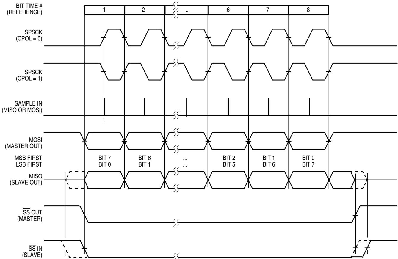
Figure 12-11. SPI Clock Formats (CPHA = 0)
