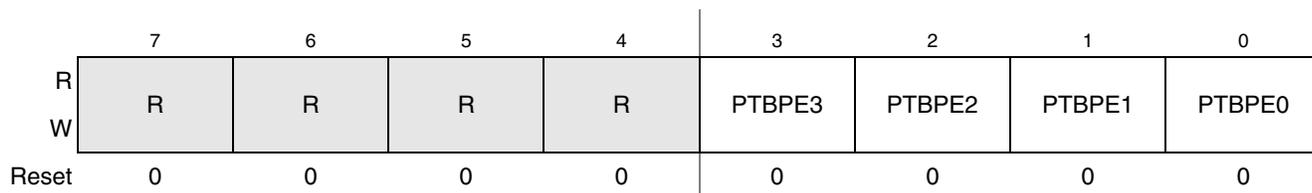
**Figure 6-17. Internal Pullup Enable for Port B (PTBPE)<sup>1</sup>**
