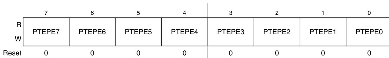
**Figure 6-32. Internal Pullup Enable for Port E (PTEPE)**
