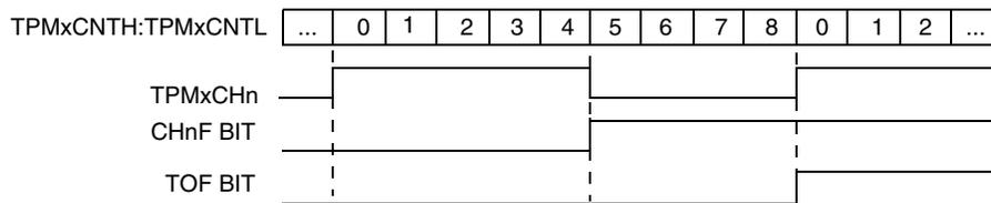
**Figure 10-3. High-True Pulse of an Edge-Aligned PWM**
