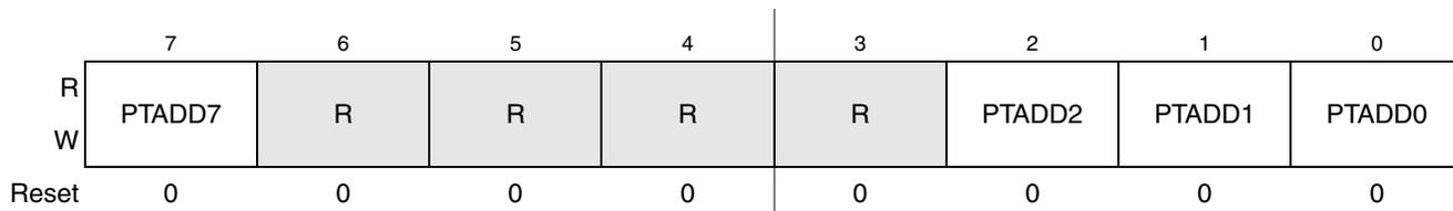
Figure 6-11. Data Direction for Port A Register (PTADD)<sup>1</sup>
