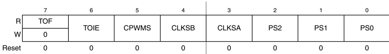
Figure 10-7. TPM Status and Control Register (TPMxSC)
