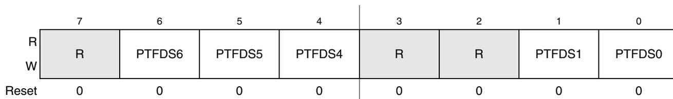
**Figure 6-39. Output Drive Strength Selection for Port F (PTFDS)<sup>1</sup>**
