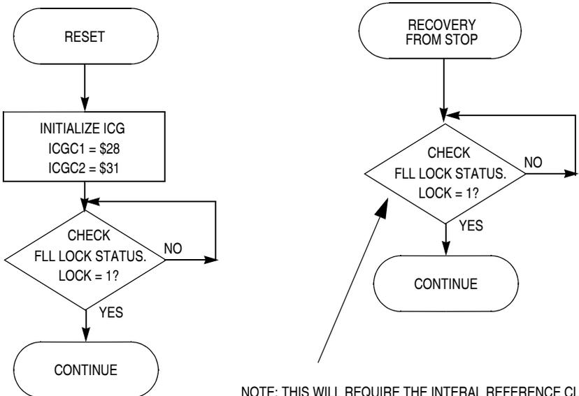
Figure 8-16. ICG Initialization and Stop Recovery for Example #3
