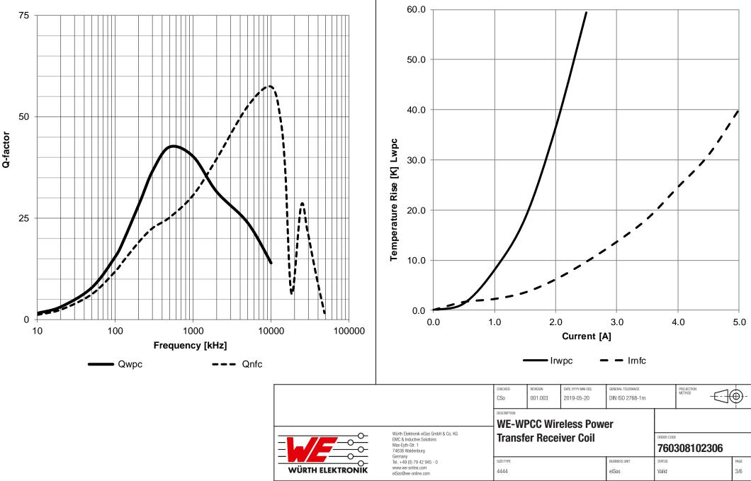
**Typical Temperature Rise vs. Current Characteristics:**
