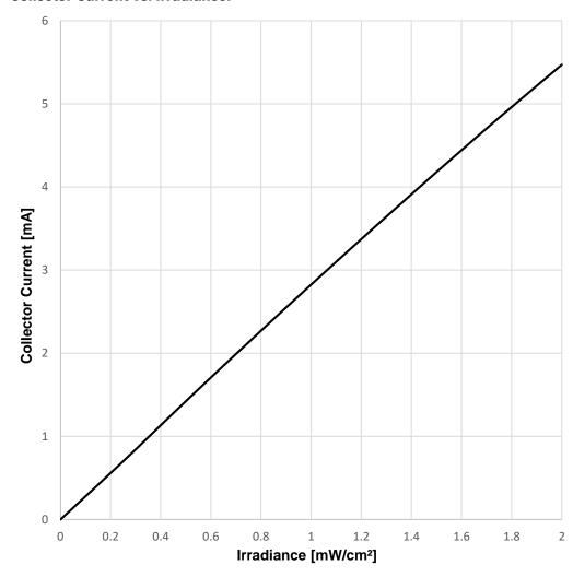
Testcondition:  $Ee = 0.5 \text{ mW/cm}^2$ , VCE = 5 V
