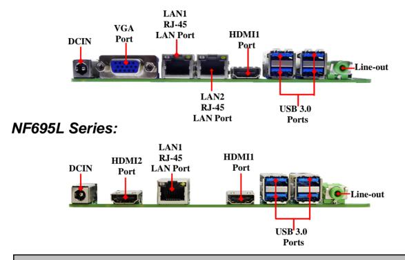
**Warning!!**The board has a 12V DC-in power connector (**DCIN3**) in I/O back panel and an internal 12V power connector (DCIN2). User can only connect one type of compatible power supply to one of them to power the system.
