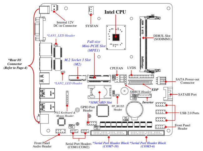
Note: SIMCARD slot only work when compatible SIM card installed & 3G LAN card installed in full-size Mini-PCIE (MPE1) slot.
