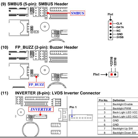
*Warning!* Find *Pin-1* location of the inverter and make sure that the installation direction is correct! Otherwise serious harm will occur to the board/display panel!!
