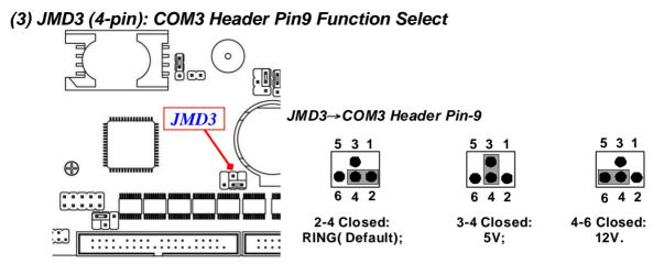
\*Note: JMD3 is only optional for NF695HV series models with COM3 serial port header(from COM3-6 combo block).
