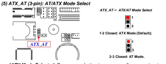
\*ATX Mode Selected: Press power button to power on after power input ready; AT Mode Selected: Directly power on as power input ready.
