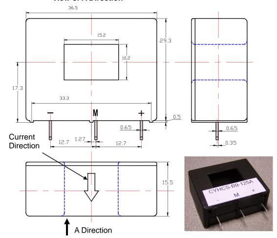
Terminal +: +12V~ 15V, Terminal -: -12V~ -15V, Terminal M: Output
