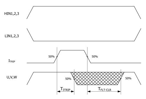
Figure 3: I<sub>TRIP</sub> Timing Waveform
