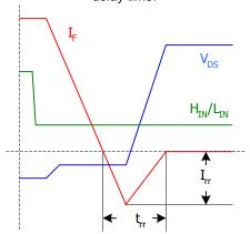
Figure 2c: Diode Reverse Recovery.
