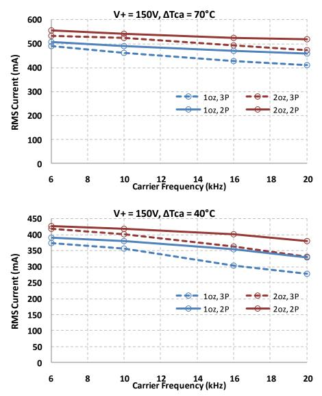
Figure 6: Maximum Sinusoidal Phase Current vs. PWM Switching Frequency Sinusoidal Modulation, V<sup>+</sup>=150V, PF=0.98
