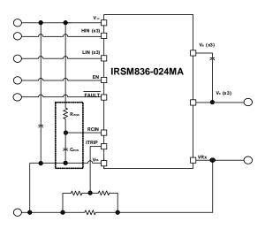
Figure 4b: Programming the fault clear timer
