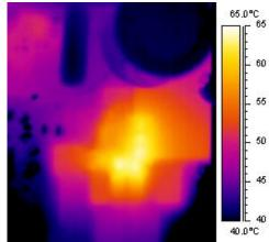
Figure 7: PCB layout example and corresponding thermal image (6kHz, 2P, 2oz, ΔTca=40°C, V+ = 150V, Iu = 427mArms, Po = 94W)
