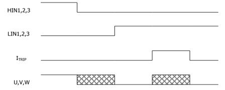
Figure 1: Input/Output Logic Diagram
