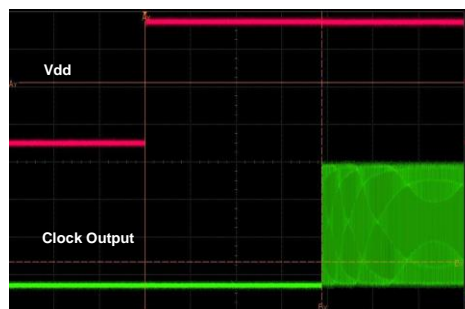
Figure 17. Startup Waveform vs. Vdd
