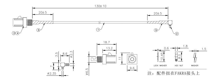
Test conditions Rated voltage: AC60V Contact Resistance:  $20m\Omega$  Withstand voltage: AC200V Insulation Resistance:  $5M\Omega$  Characteristic impedance:  $50\Omega$
