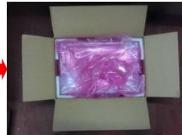
Then put anti-static bag into carton which has EPE cushion in it
