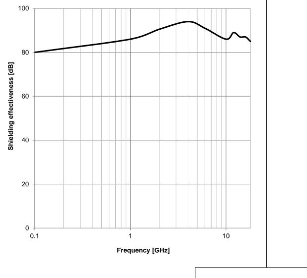
CHECKED REVISION DATE (YYYY-MM-DD) GENERAL TOLERANCE PROJECTION METHOD ViMa 004.003 2020-03-06 DIN ISO 2768-1m DESCRIPTION **WE-LT Conductive Shielding** Würth Elektronik eiSos GmbH & Co. KG Gasket ORDER CODE EMC & Inductive Solutions Max-Eyth-Str. 1 302064032 74638 Waldenburg Germany SIZE/TYPE STATUS Tel. +49 (0) 79 42 945 - 0 www.we-online.com BUSINESS UNIT PAGE WÜRTH ELEKTRONIK 2/3 eiSos Valid Square eiSos@we-online.com
