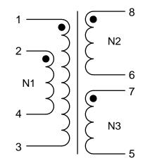
N1 denotes two windings connected in parallel. Terminals 1+2 and 3+4 must be tied as solder bridging is allowed.
