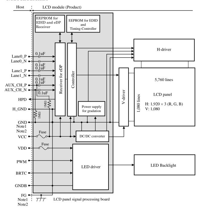
Note1: Relations between H\_GND (High Speed Ground), GND (Signal ground), GNDB (LED driver ground) and FG (Frame ground) in the LCD module are as follows.
