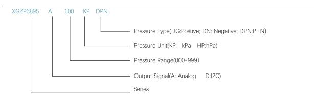
Note: 1. Voltage 5Vdc as default value, add 33 behind mode signify 3.3V power supply, e.g.: XGZP6895A050KPDG33.
