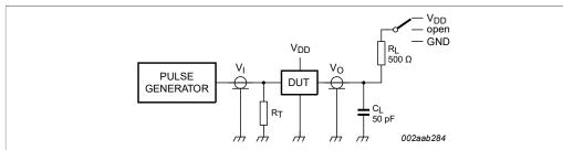
$R_L$  = Load resistor for LEDn.  $R_L$  for SDA and SCL > 1 k $\Omega$  (3 mA or less current).
