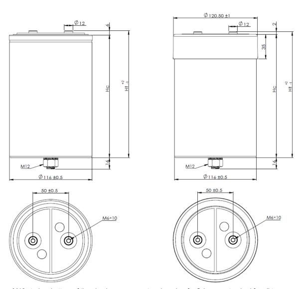
M12 stud on bottom of the aluminum case, nut and washer for fixing are standard for all types.
