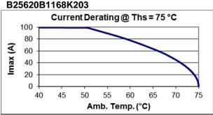
Current derating graphs are based on typical values. Graphs for capacitors rated 1320 / 1500/2000 **U**<sub>NDC</sub> are available upon request.
