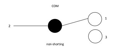
Type of Schematic: SPDT
