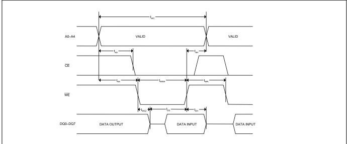
Figure 3. Write Cycle Timing, Chip-Enable Controlled
