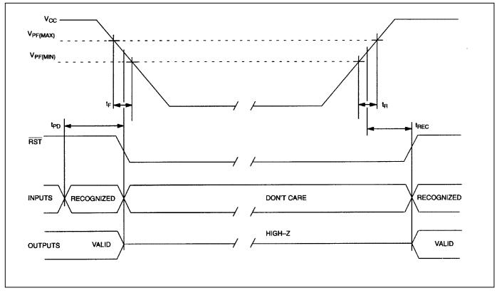
Figure 5. 3.3V Power-Up/Down Waveform Timing
