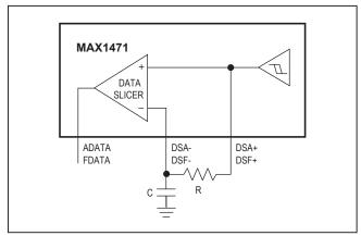
Figure 4. Generating Data-Slicer Threshold Using a Lowpass Filter
