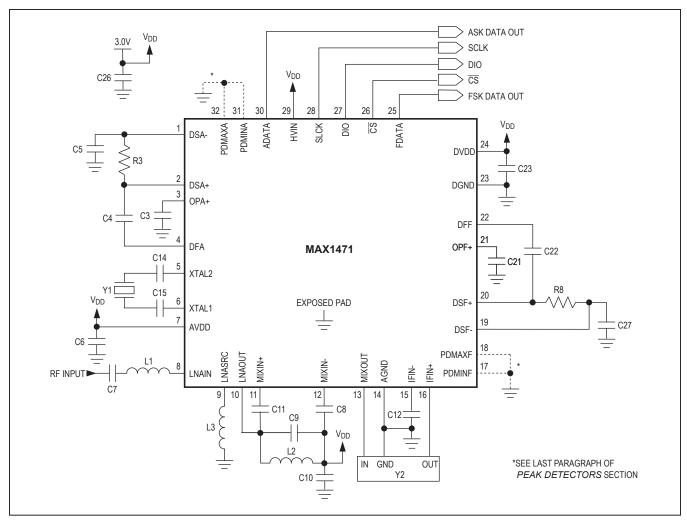
Figure 2. Typical Application Circuit
