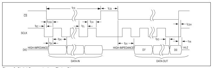
Figure 8. Digital Communications Timing Diagram
