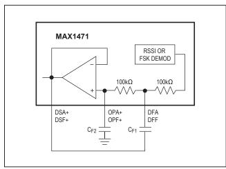
Figure 3. Sallen-Key Lowpass Data Filter
