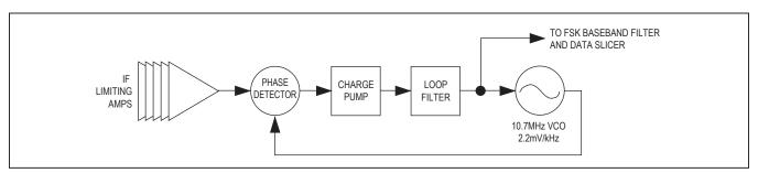
Figure 1. FSK Demodulator PLL Block Diagram
