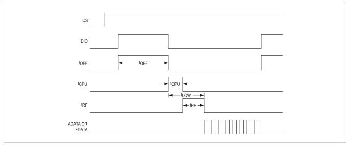
Figure 12. DRX Mode Sequence of the MAX1471
