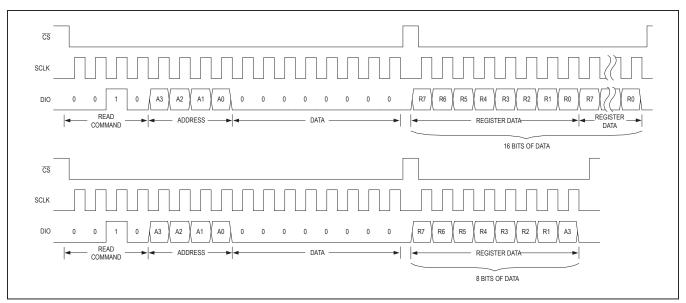
Figure 11. Read Command in 3-Wire Interface
