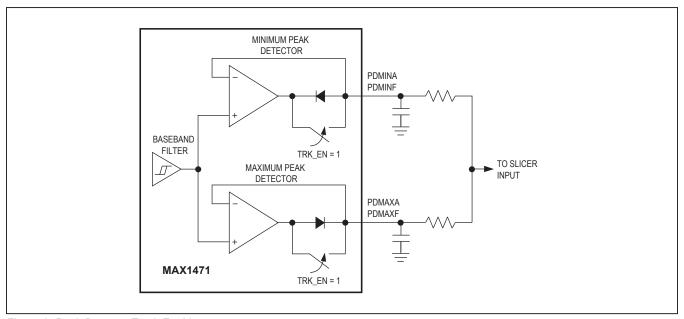
Figure 6. Peak-Detector Track Enable
