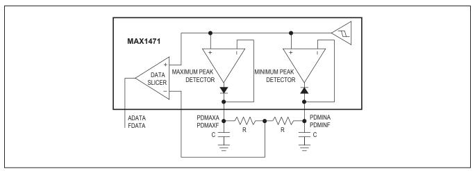
Figure 5. Generating Data-Slicer Threshold Using the Peak Detectors
