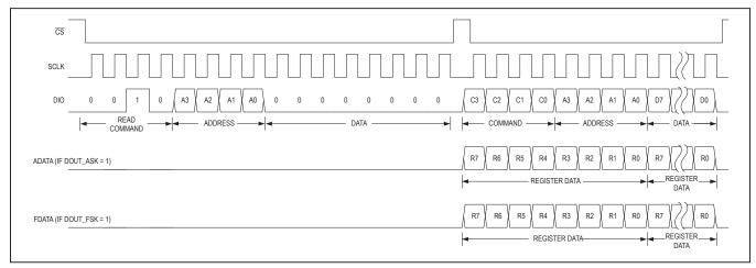
Figure 10. Read Command on a 4-Wire SERIAL Interface
