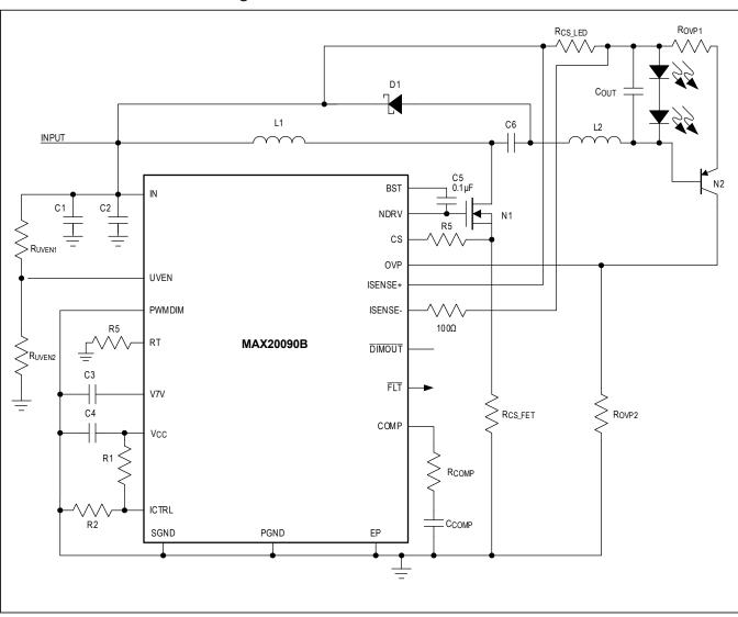
**Ćuk Converter LED Driver using the MAX20090**
