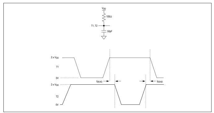
Figure 1. T1, T2 Timing Diagram
