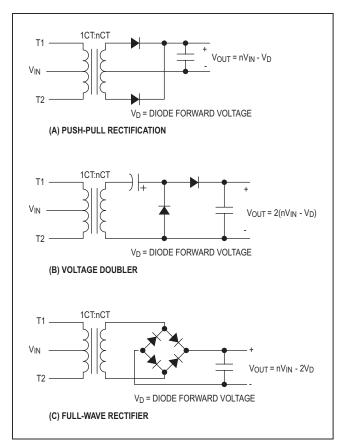
Figure 2. Secondary-Side Rectification Topologies
