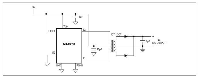
Figure 3. 5V to Isolated, Unregulated 6V Application Circuit
