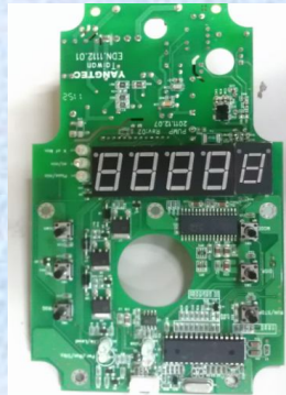
← Pump Controller Board
